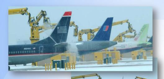
A number of projects at PHL and PNE help improve water quality and protect existing wetlands. PHL's centralized deicing facility captures and disposes of deicing fluid runoff properly to protect nearby waterways and groundwater. PHL also eliminated urea-based deicing products used on runway and taxiway pavement areas to reduce water pollution and algae growth in surrounding waterways that lead to the Delaware River.
