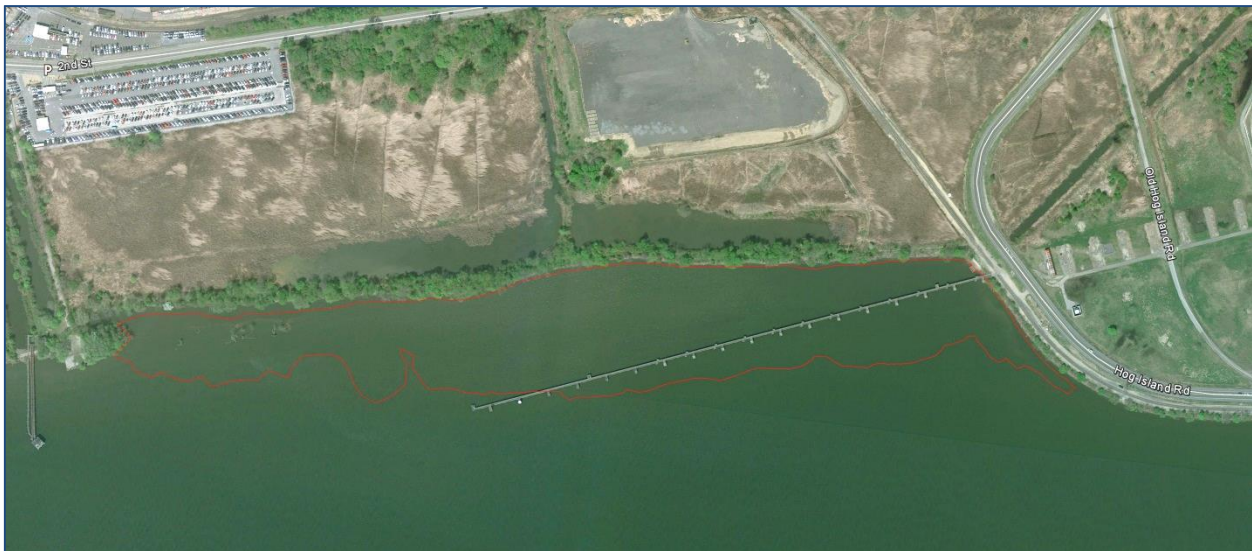
Aerial 2: Project area tidal wetlands covered at high tide. (Source: Google Earth 4/11/2010) Mean high water is at elevation +3.16. Tide range is 5.52 feet.
